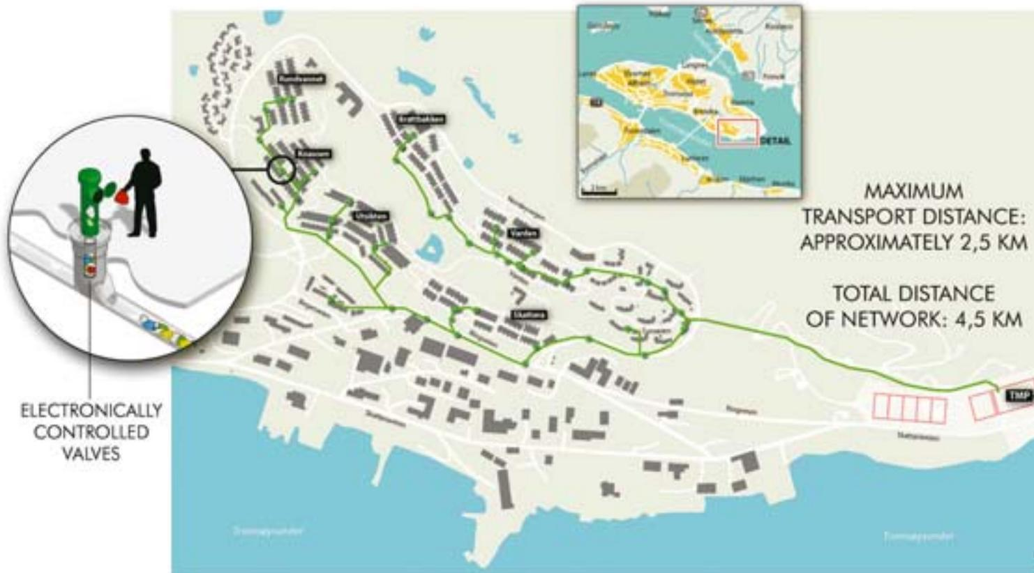
problems now. I also want to emphasise the enormous improvement this will have on the living environment in Stakkevollan. All waste containers have now been replaced with indoor or outdoor inlet so all waste is automatically transported down to the underground optical waste sorting installation. This means we no longer need sanitation trucks in the area. It has been very exciting to work on this environment and engineering project” says Bård Jørgensen in closing.
