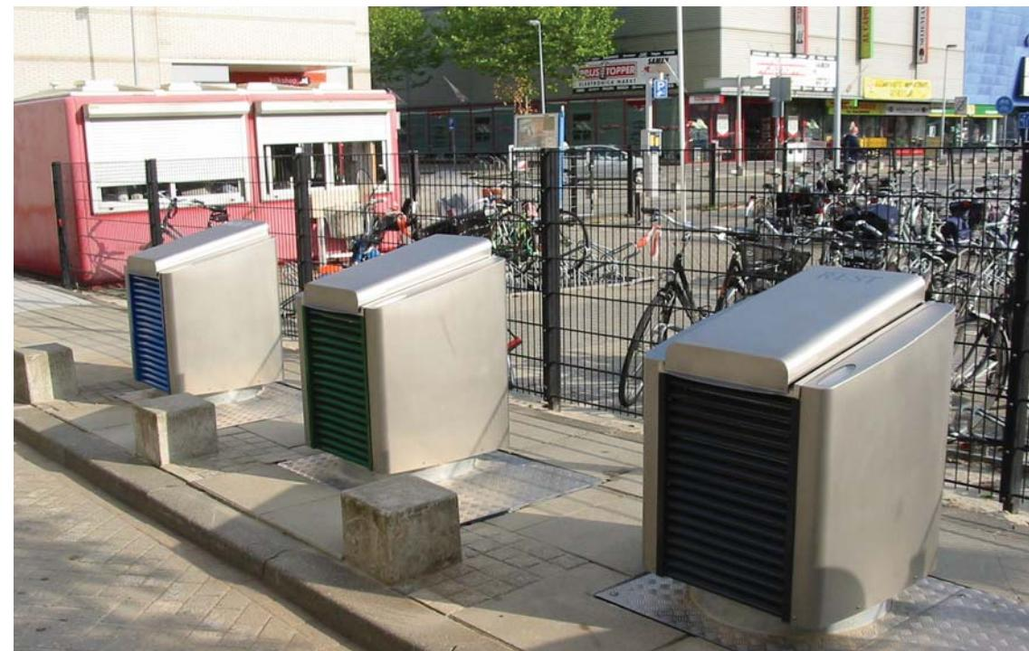
Separate waste inlets for 3 waste fractions.
