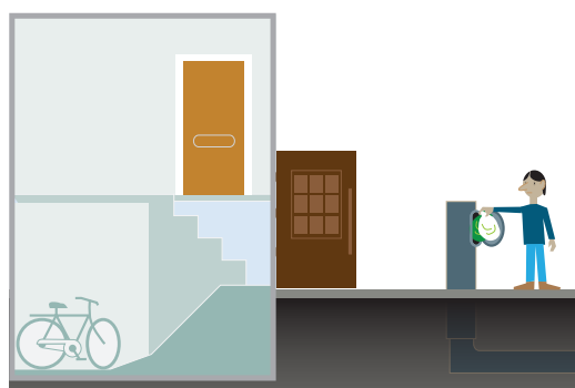
Waste collection with pneumatic waste systems frees up space and provides a better working environment.
